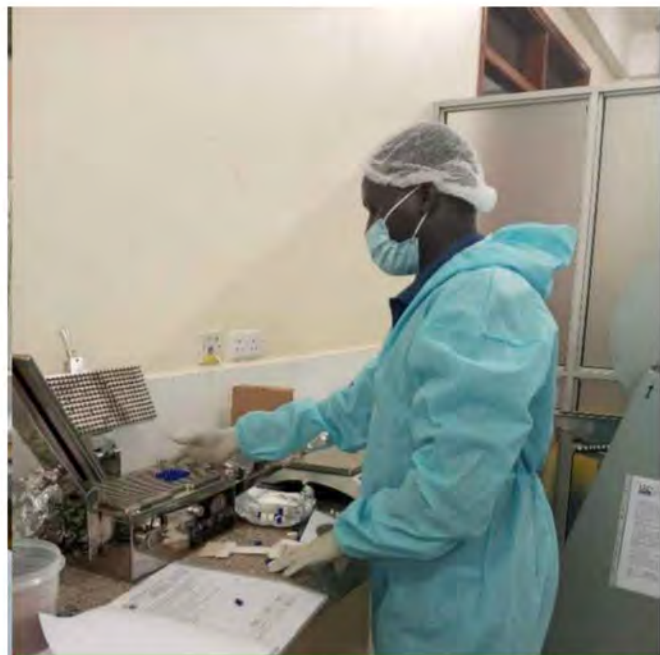
Development of herbal capsule formulation using semi-automated equipment
