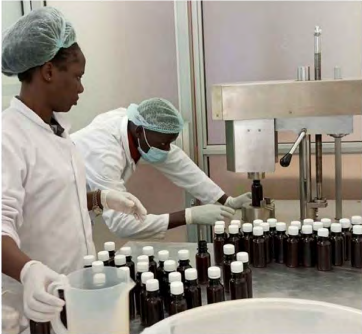
The PHARMBIOTRAC Product Development Officer Mr. Jimmy Angupale in the PHARMBIOTRAC production lab demonstrating to students of Mbarara University of Science and Technology, Uganda on how to cap syrup bottles using a semi-automated capping machine.
